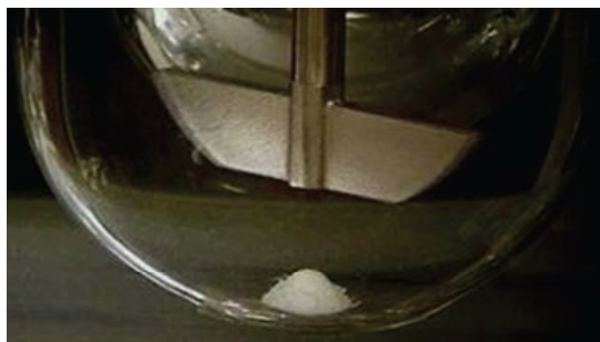
Figure 3: Operation of a paddle apparatus set at 50 rpm with a USP prednisone performance tablet highlighting the flaw of poor stirring and mixing environment within a dissolution vessel causing incorrect characterization of dissolution/quality attribute of the product.
