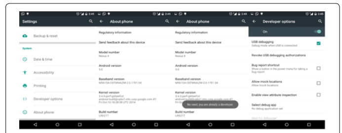
Figure 5: Enabling USB debugging on Android device.
