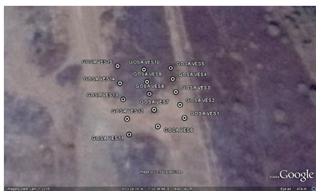
Figure 3: Google Earth map showing the VES points for the open dumpsite in Gosa, Abuja.
