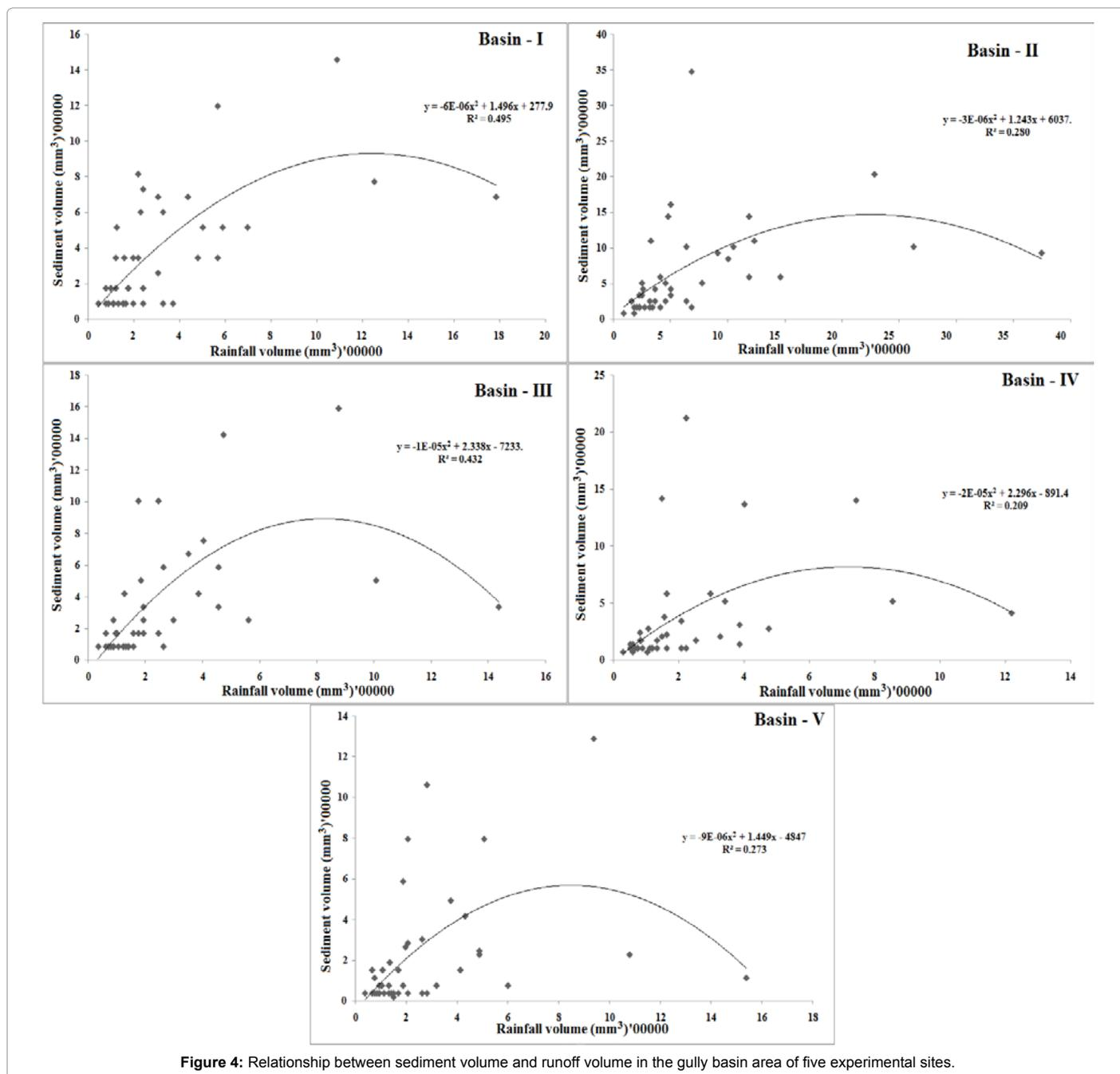
Figure 4: Relationship between sediment volume and runoff volume in the gully basin area of five experimental sites.
