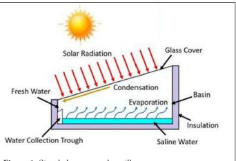
Figure 1: Simple box type solar still.
