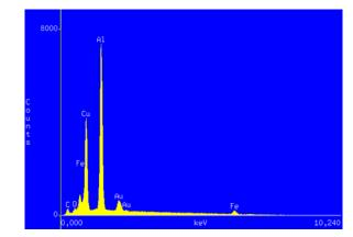
Figure 3b: EDS elemental analysis of quasicrystalline alloy Al<sub>62,2</sub>Cu<sub>25,3</sub>Fe<sub>12,5</sub> showing the icosahedral phase after heat treatment at 8 h.
