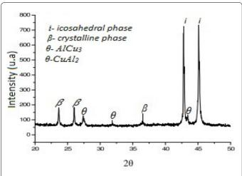
Figure 1: X-Ray diffraction (XRD) of the sample  $Al_{_{82,2}}Cu_{_{25,3}}Fe_{_{12,5}}$  heat treated in time of 8 h.
