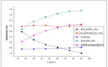
Figure 7: Catalytic behavior of the sample quasicrystal  $AI_{62,2}Cu_{25,3}Fe_{12,5}$  on the basis of selectivity (%) of the product and time in minutes.
