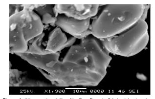
Figure 4: Alloy quasicrystalline Al<sub>62,2</sub>Cu<sub>25,3</sub>Fe<sub>12,5</sub> to 8 h heat treatment and subjected to a catalytic reaction.
