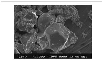
Figure 3a: Image quasicrystalline the surface of the alloy Al<sub>62.2</sub>Cu<sub>25.3</sub>Fe<sub>12.5</sub> showing the icosahedral phase, at 8 h.
