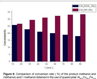
methanolic acid + methanol obtained in the use of quasicrystal  $Al_{62,2}Cu_{25,3}$ Fe as a catalyst versus time (minutes).
