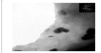
Figure 6: Image Transmission Electron Microscopy - MET league of quasicrystalline  ${\rm AI}_{\rm 622}{\rm Cu}_{25.3}{\rm Fe}_{12.5}$  after a catalytic reaction.
