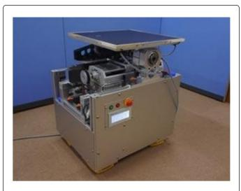
Figure 1: The new type of dynamic trunk balance evaluator
