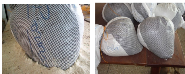
Plate 4: Effect of LGB on the polypropylene and hermetic bags after 6 mo.
