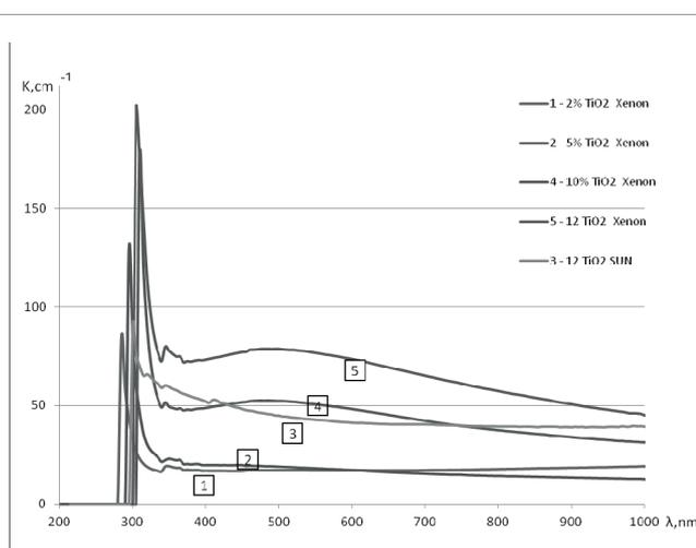
**Figure 5:** Absorption spectra of cordierite glasses doped by  $\text{TiO}_2$  syntheses by irradiation of: Xenon lamp (curves 1, 2, 4, 5), Sun (curve 3).
