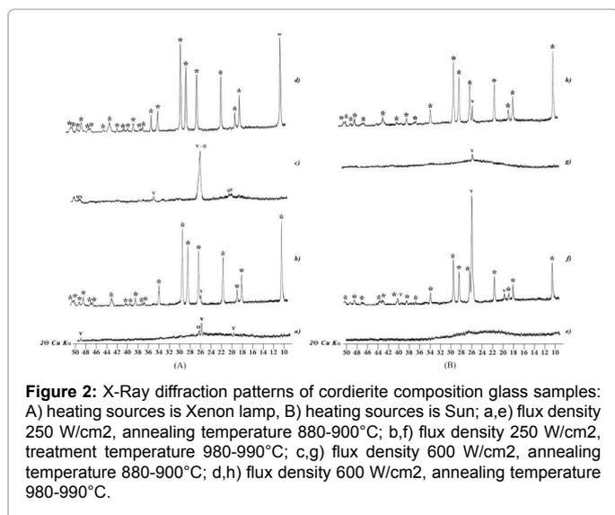
Figure 2: X-Ray diffraction patterns of cordierite composition glass samples: A) heating sources is Xenon lamp, B) heating sources is Sun; a,e) flux density 250 W/cm<sup>2</sup>, annealing temperature 880-900°C; b,f) flux density 250 W/cm<sup>2</sup>, treatment temperature 980-990°C; c,g) flux density 600 W/cm<sup>2</sup>, annealing temperature 880-900°C; d,h) flux density 600 W/cm<sup>2</sup>, annealing temperature 980-990°C.
