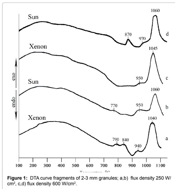
Figure 1: DTA curve fragments of 2-3 mm granules; a,b) flux density 250 W/cm<sup>2</sup>, c,d) flux density 600 W/cm<sup>2</sup>.
