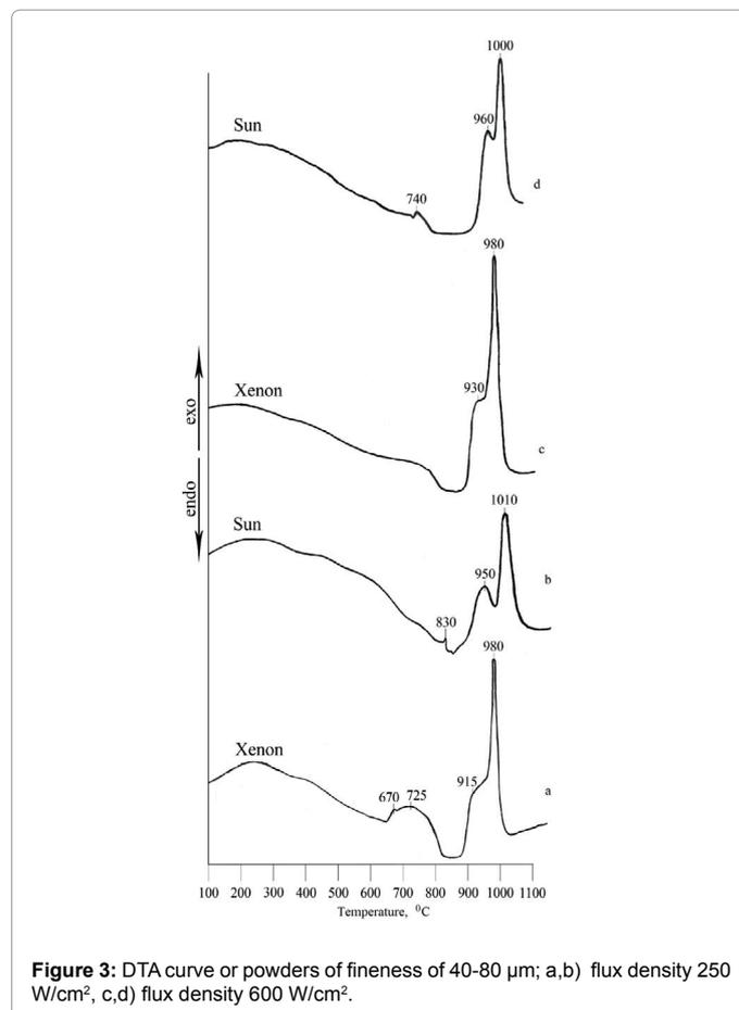
Figure 3: DTA curve of powders of fineness of 40-80  $\mu m$ ; a,b) flux density 250 W/cm<sup>2</sup>, c,d) flux density 600 W/cm<sup>2</sup>.
