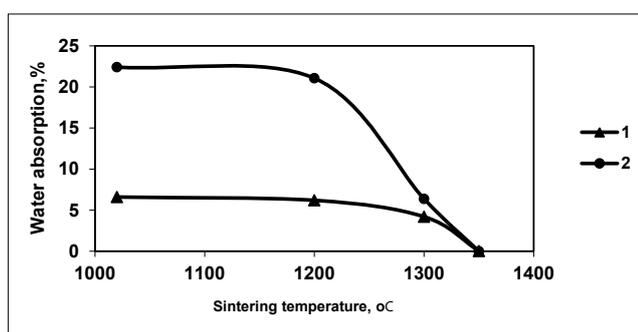
**Figure 4:** The dependence of the degree of sintering of cordierite glass composition with the addition of 12 wt %  $\text{TiO}_2$  on synthesis conditions, the melt holding time is 5 minutes: 1) of a Xenon lamp; 2) the solar radiation.
