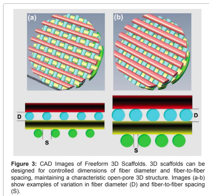
Figure 3: CAD Images of Freeform 3D Scaffolds. 3D scaffolds can be designed for controlled dimensions of fiber diameter and fiber-to-fiber spacing, maintaining a characteristic open-pore 3D structure. Images (a-b) show examples of variation in fiber diameter (D) and fiber-to-fiber spacing (S).
