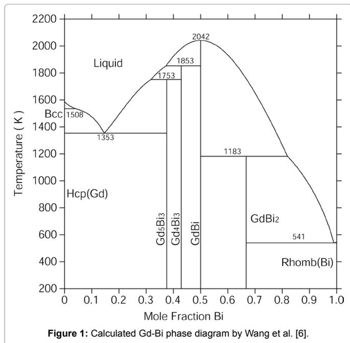
Figure 1: Calculated Gd-Bi phase diagram by Wang et al. [6].
