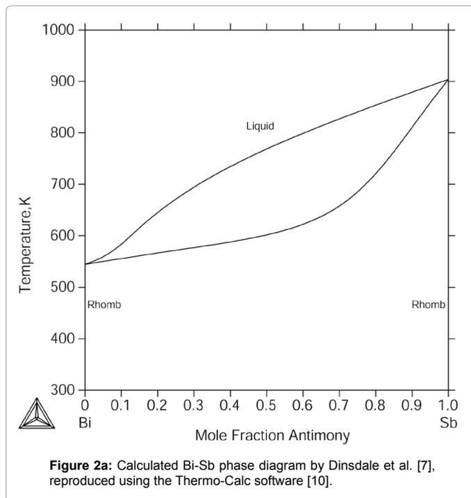
Figure 2a: Calculated Bi-Sb phase diagram by Dinsdale et al. [7], reproduced using the Thermo-Calc software [10].
