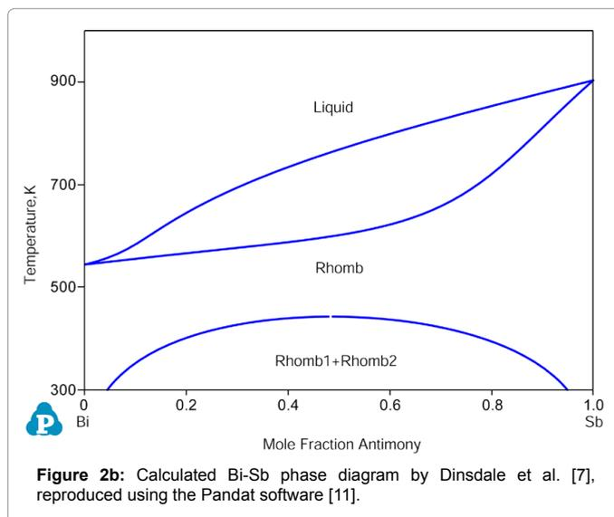
Figure 2b: Calculated Bi-Sb phase diagram by Dinsdale et al. [7], reproduced using the Pandat software [11].
