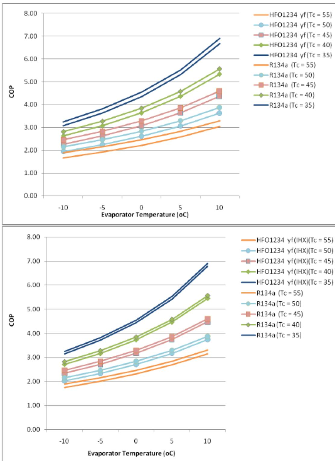
Figure 8: Theoretical COP Vs. Evaporator Temperature (At varying condenser temp) (with and without heat exchanger).
