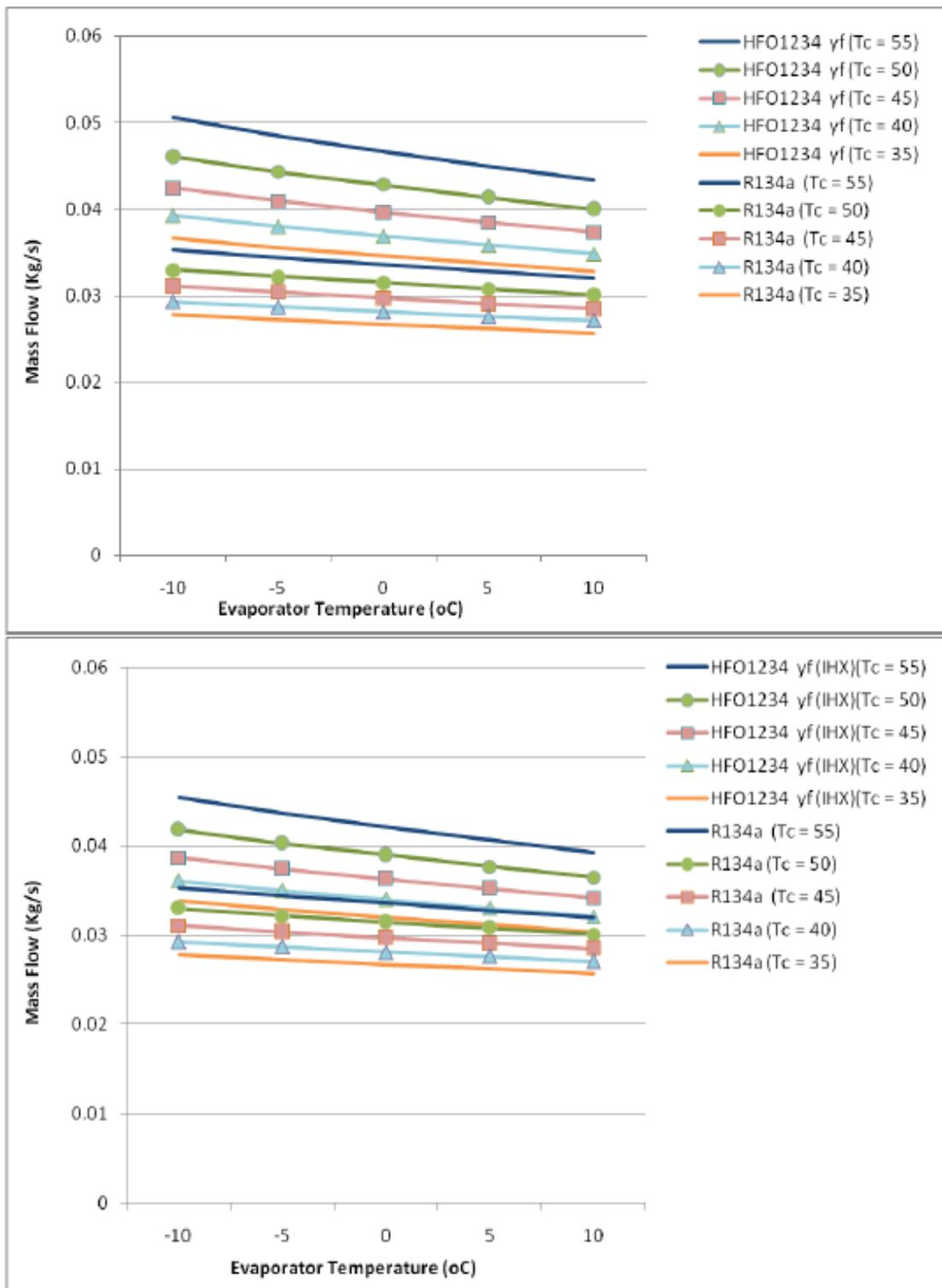
Figure 6: Theoretical Mass flow rate Vs. Evaporator Temperature (At varying condenser temp) (with and without heat exchanger).
