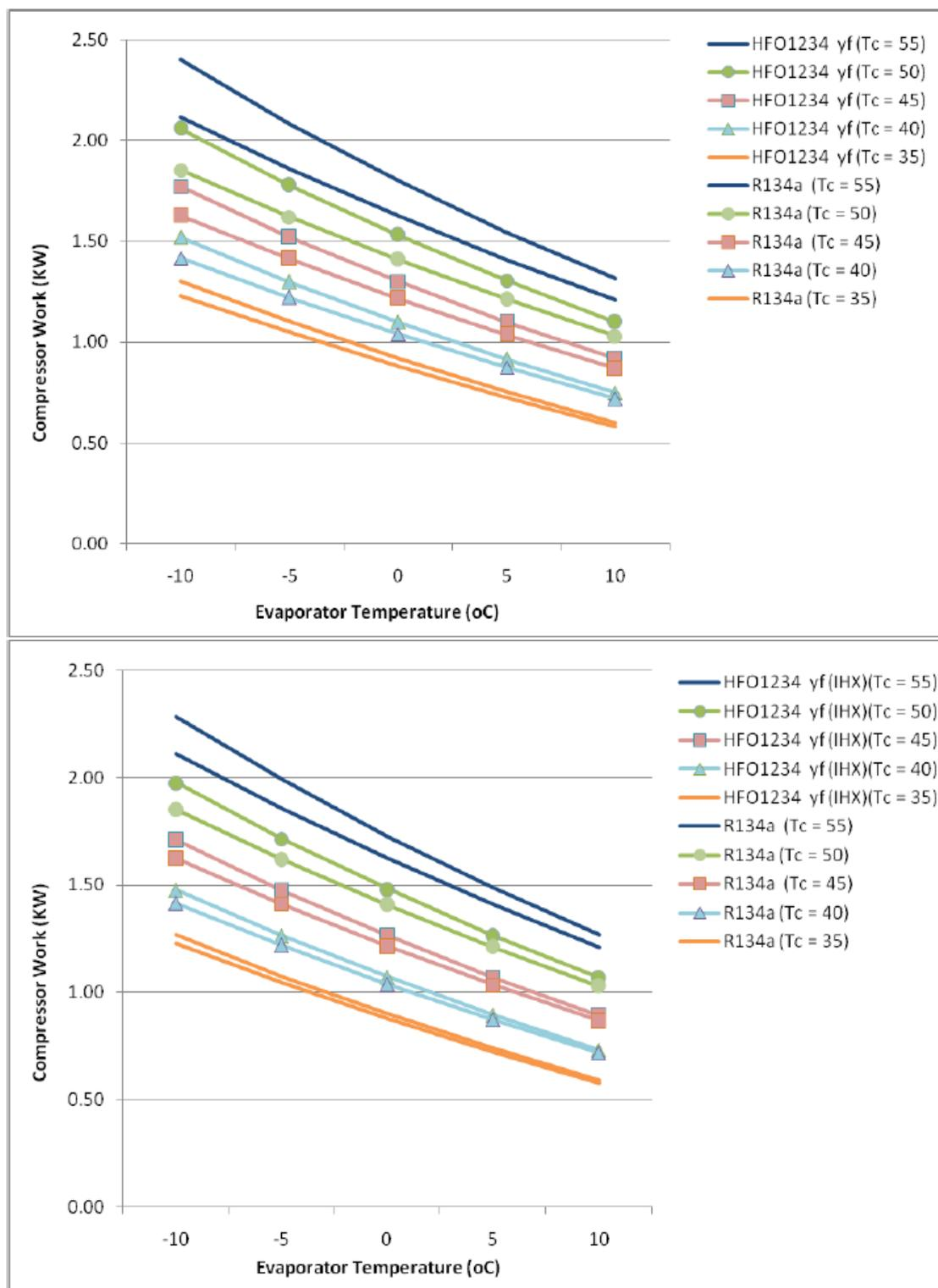
Figure 7: Theoretical Compressor work Vs. Evaporator Temperature (At varying condenser temp) (with and without heat exchanger)
