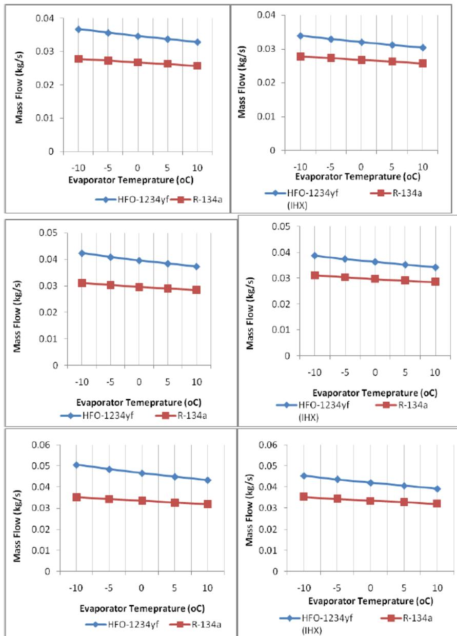
Figure 3: Mass flow rate Vs. Evaporator temperature at condensation temp 35°C A) without IHx, B) With IHx, at condensation temp 45°C C) Without IHx & D) With IHx and at condensation temp 55°C E) Without IHx and F) With IHx.
