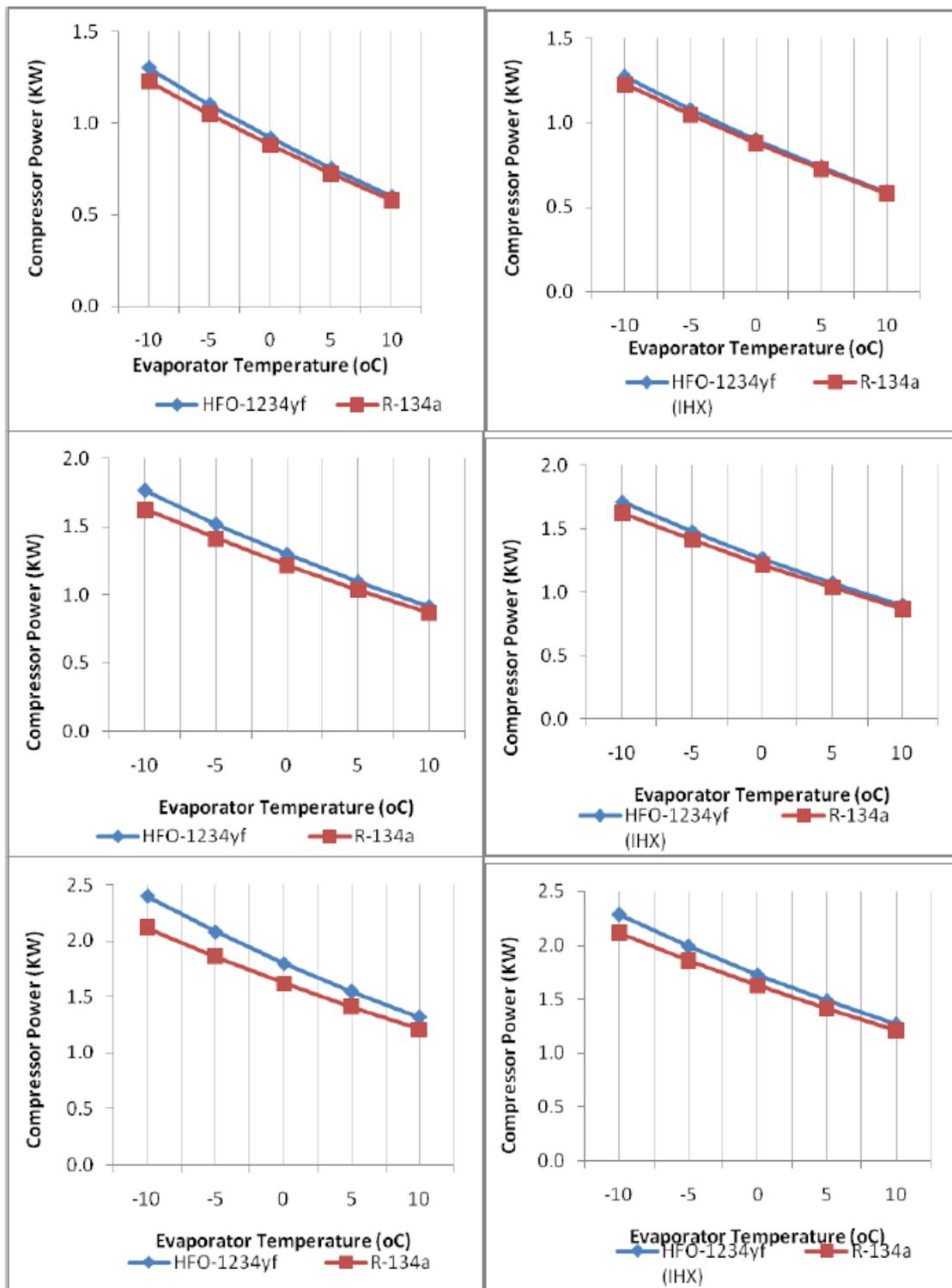
Figure 4: Compressor Work Vs. Evaporator Temperature at condensation temp 35°C A) Without IHX, B) With IHX, at condensation temp 45°C, C) Without IHX and D) With IHX and at condensation temp 55°C E) Without IHX and F) With IHX
