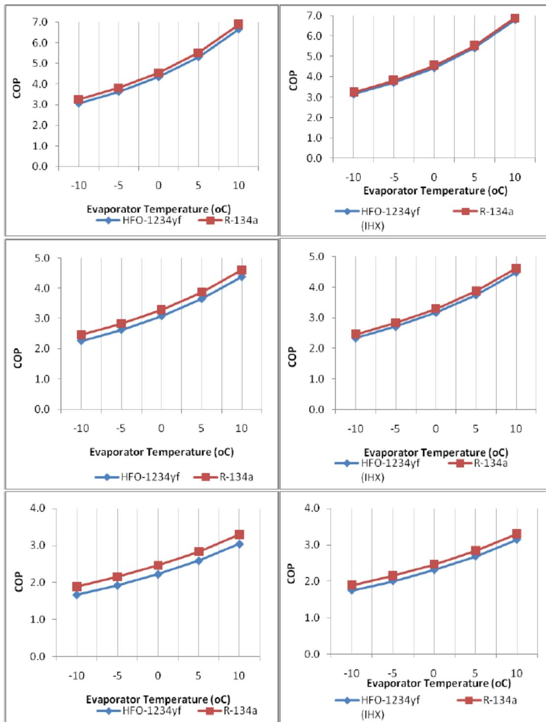
Figure 5: COP Vs. Evaporator Temperature at condensation temp 35°C A) Without IHX, B) With IHX, at condensation temp 45°C C) Without IHX & D) With IHX and at condensation temp 55°C E) Without IHX and F) With IHX.
