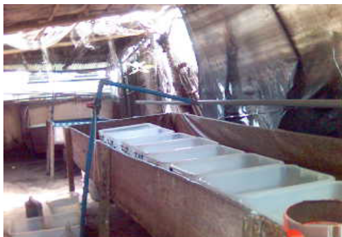
Figure 2: Culture tanks enclosed in a bath tub.
