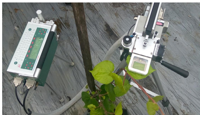
Figure 1: Measurement photosynthesis rate, stomatal conductance, and transpiration rate by Li-Cor 6400 Portable Photosynthesis system.
