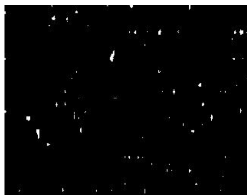
Figure 8: The microstructure of the surface of the stainless steel electrode with a thin layer (d=15 μm) of chromium after its operation 45 h.
