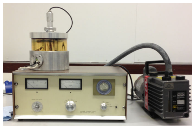
Figure 3: Gold coating machine at London South Bank University SEM laboratory.
