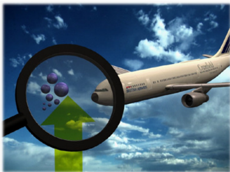
Figure 1: Various super-cooled droplet sized encounters in presence of a rising air system and high humidity resulting in aircraft icing [3].
