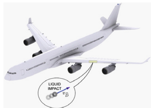
Figure 2: A possible impact scenario, with liquid impacts ensuing in either splashing, ice adhesion or erosion [5].
