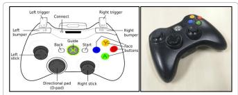
Figure 7: Xbox 360 wireless controller, Manufacturer: Microsoft, Release year: 2005.
