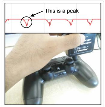
Figure 17: Force meter graph for buttons.
