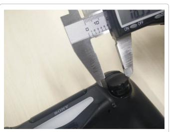
Figure 12: Face button measurement.
