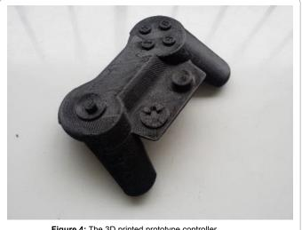
Figure 4: The 3D printed prototype controller.
