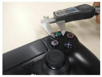
Figure 3: Measuring the diameter of the face buttons.
