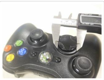
Figure 13: Diameter of the directional pad.
