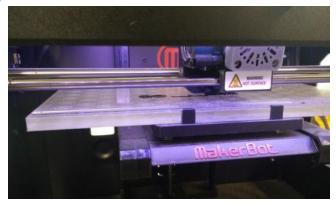
Figure 24: 3D printing: Prototype controller.
