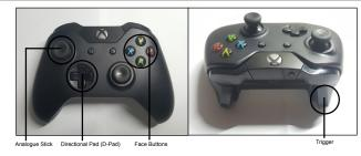
Figure 9: General components of a controller.
