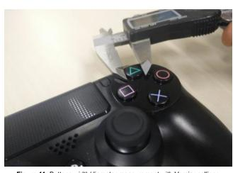
Figure 11: Buttons width/diameter measurement with Vernier calliper.
