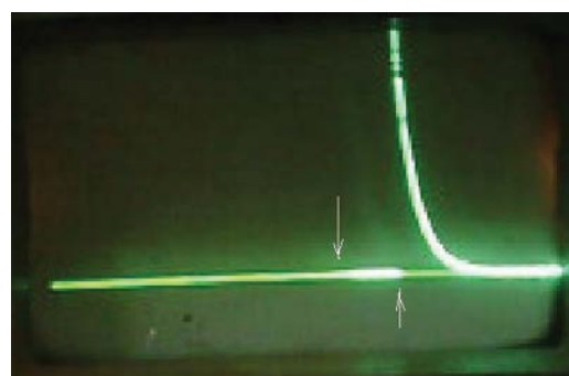
Figure 7: Oscilloscope trace of the electric current during the explosion in air. The white arrows indicate the beginning and end of the induction period.
