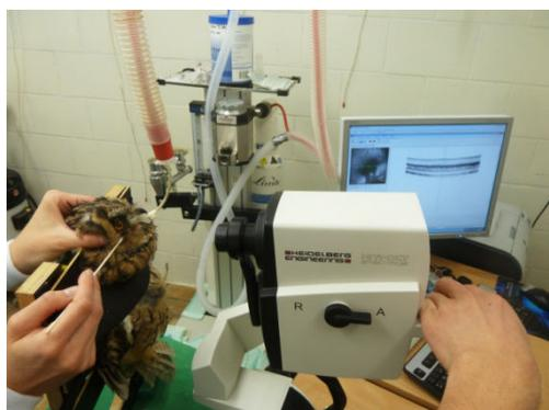
**Figure 1:** Photograph of the OCT device, fixation plate and anesthesia circuit used in this study. In this picture a long-eared owl (*Asio otus*) is under examination. The bird was anesthetized, and only one person was holding the plate and the animal's head, and kept the eyelid open. The original distance of the OCT lens during the volume scan was smaller.
