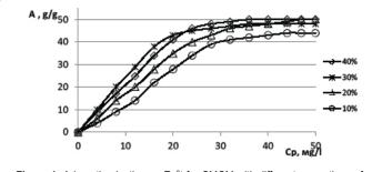
Figure 1: Adsorption isotherms  $\mathsf{Zn}^{2*}$  for CMCM with different proportions of HTMT additive.
