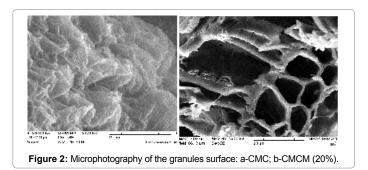
Surface morphology analysis of CMCM containing HTMT 20% and without it revealed that with HTMT additive appears porous surface area. Porous structure of the surface results from the increase of CMCM sorption capacity with HTMT additive.
