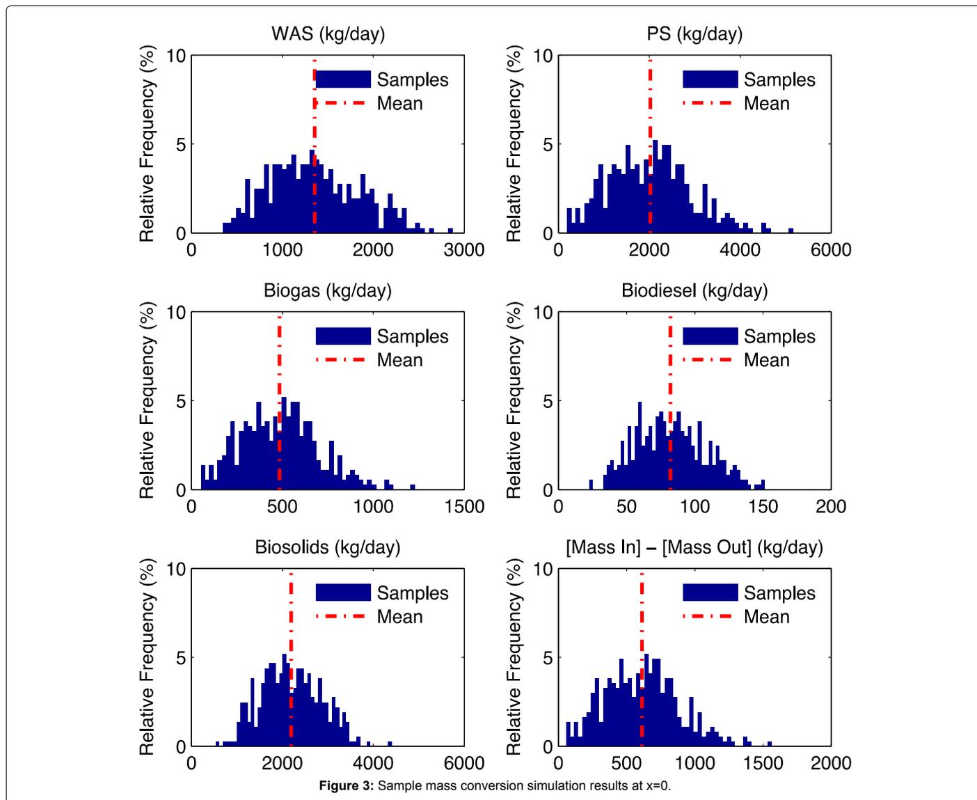
**Figure 3:** Sample mass conversion simulation results at x=0.
