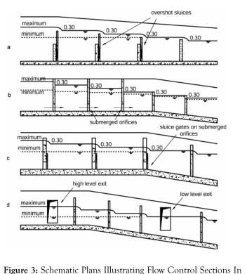
**Figure 3:** Schematic Plans Illustrating Flow Control Sections In Fishway [9]; Note, dimensions are in metric.
