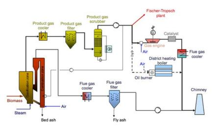
(i) The flue gas is cooled, cleaned of ash and released into the atmosphere by a chimney as above. (ii) Bed ash and fly ash could be sold to construction materials manufacturing sector whilst (iii) CO and CO2 emissions from chimney are monitored. (iv) Dry hot gas and wet cooled gas cleaning [7] are used with the Fischer-Tropsch synthesis to biofuels (Figure 3).
