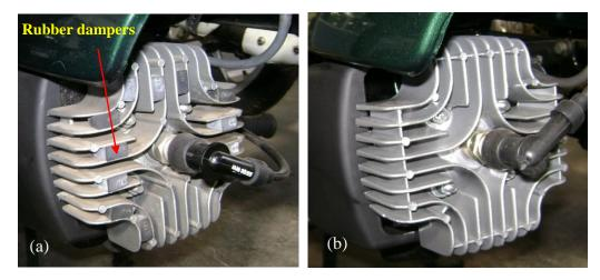
Figure 1: (a) Old engine with rubber dampers, (b) new engine without rubber dampers.
