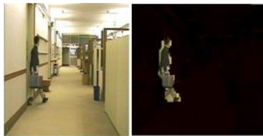
Fig. 3: Example of Compressed Domain Object Segmentation
