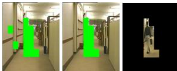
Fig. 2: Example of Compressed Domain MV Noise Filtering
