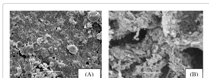
**Figure 5:** SEM micrographs of HA agglomerates in the composite membranes.
