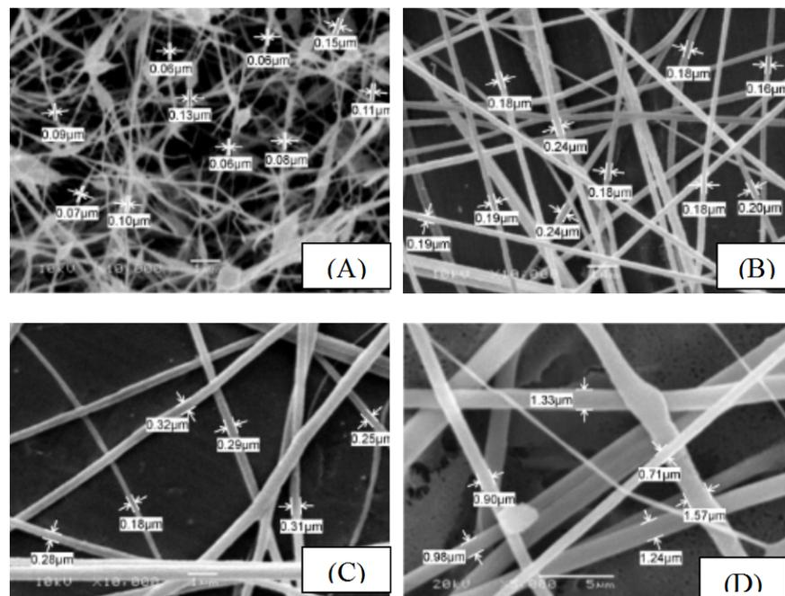
Figure 2: SEM images of the electrospun polymeric nanofibrous membranes.
