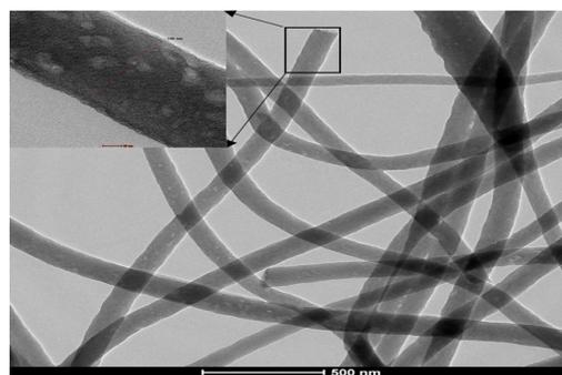
Figure 4: High resolution-TEM images of the prepared CNFs membranes after hydrothermal processing.
