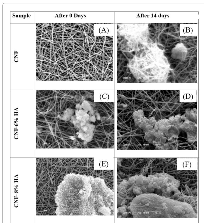
**Figure 6:** (A) SEM images of CNF, CNF-6% HA, and CNF-8%HA composite nanofibers before and after immersion into SBF solution for 14 days; (B) SEM images taken after 14 days which revealed the intense formation of the apatite-like materials throughout the CNFs membranes.
