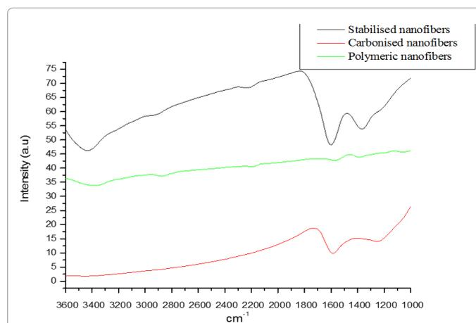
Figure 3: The difference of the functional groups before and after the heat treatment of the polymeric nanofiber by FT-IR analysis.
