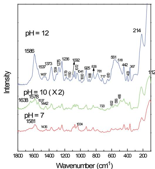
Figure 4: SERS of diclofenac (in methanol)  $10^{-3}$  M on Ag colloid+KNO<sub>3</sub>  $10^{-2}$  M at different pH.
