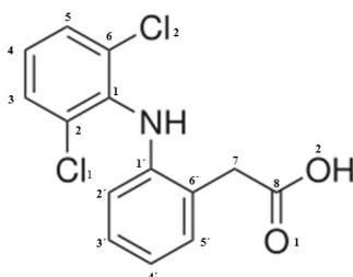
Figure 1: Structure of diclofenac.
