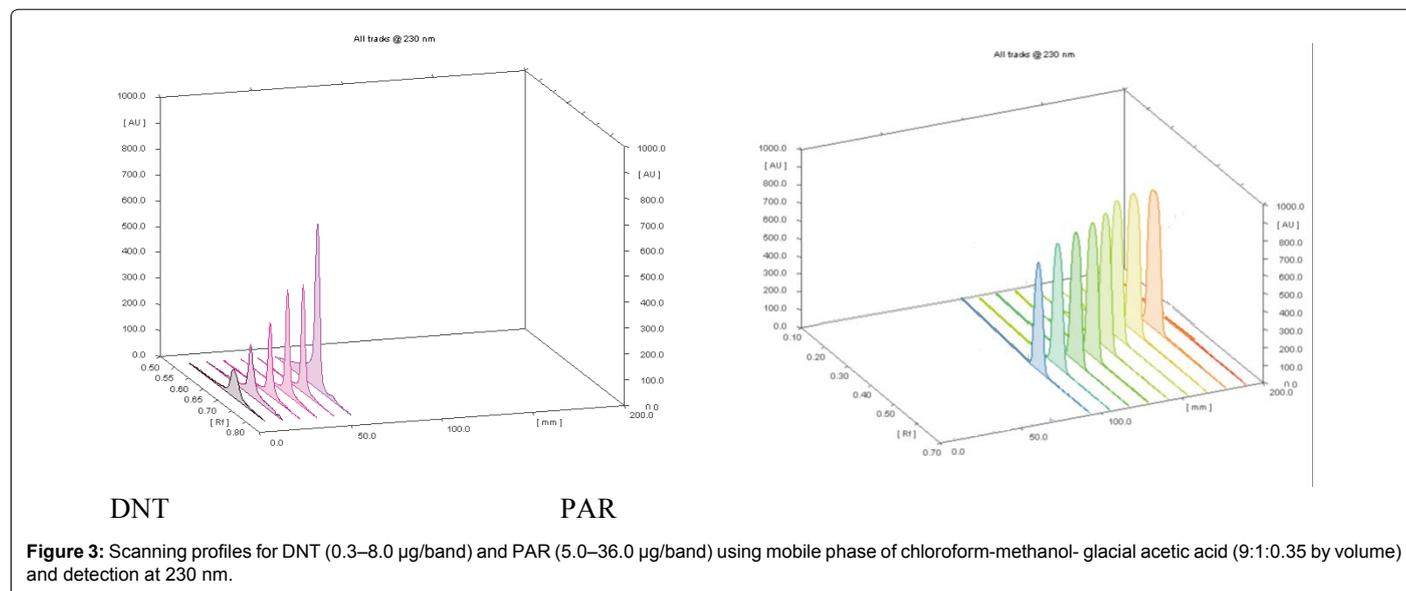
Figure 3: Scanning profiles for DNT (0.3–8.0 µg/band) and PAR (5.0–36.0 µg/band) using mobile phase of chloroform-methanol- glacial acetic acid (9:1:0.35 by volume) and detection at 230 nm.
