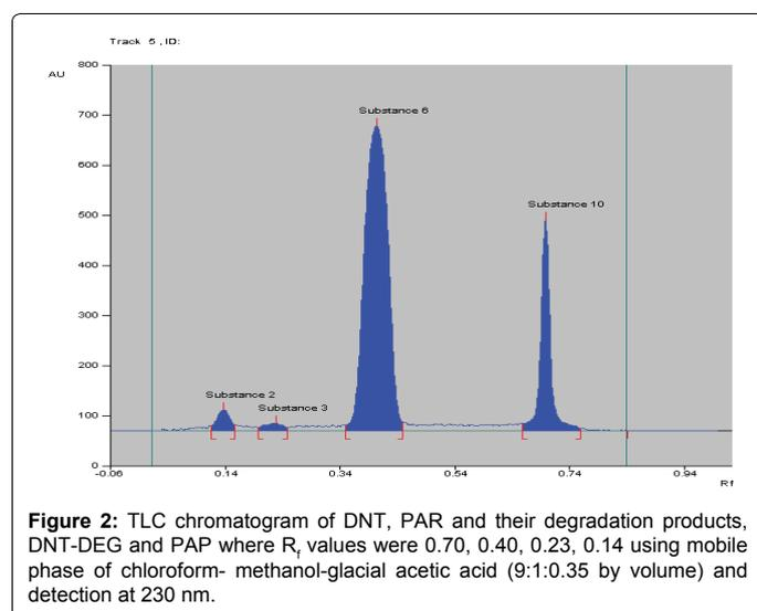
**Figure 2:** TLC chromatogram of DNT, PAR and their degradation products, DNT-DEG and PAP where  $R_f$  values were 0.70, 0.40, 0.23, 0.14 using mobile phase of chloroform- methanol-glacial acetic acid (9:1:0.35 by volume) and detection at 230 nm.
