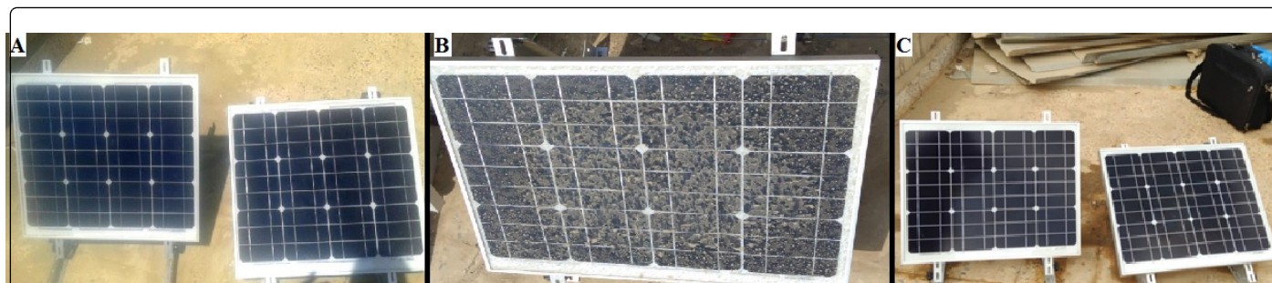
Figure 3: A. Solar cells state at the beginning of measurement; B. After a weak rainfall; C. After cleaning by smooth normal water.
