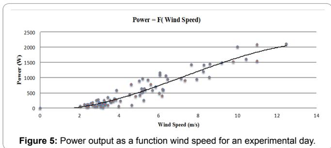
Figure 5: Power output as a function wind speed for an experimental day.
