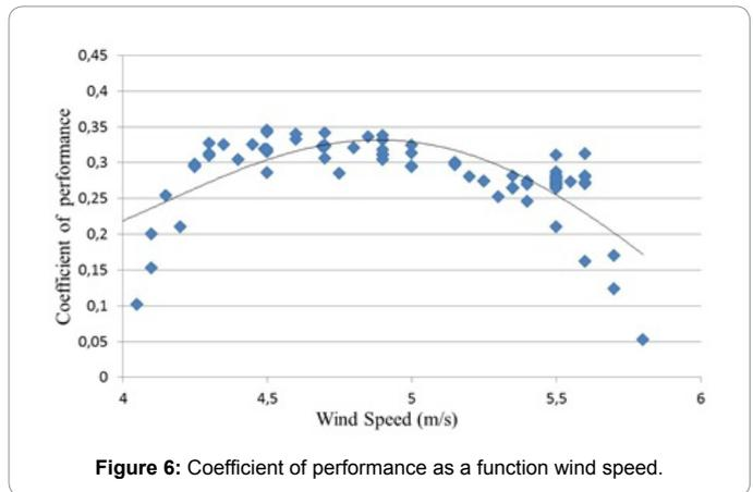
Figure 6: Coefficient of performance as a function wind speed.
