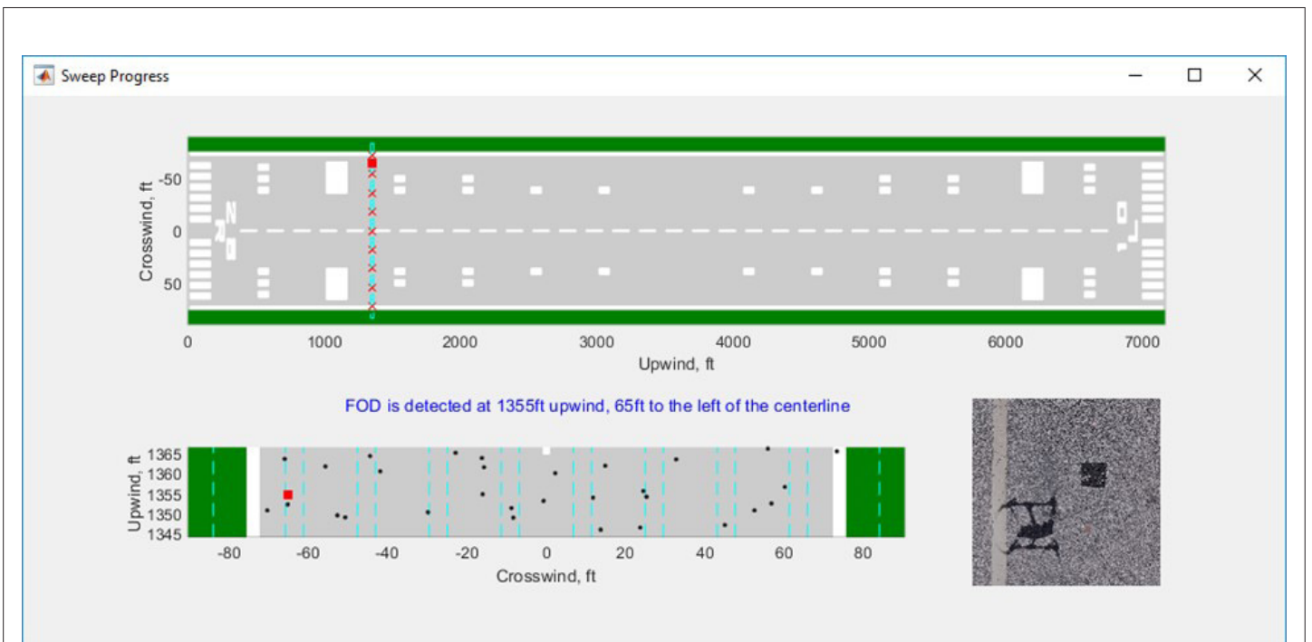
Figure 5: Detachable window showing the image of a detected FOD candidate.
