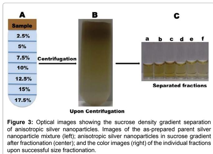
**Figure 3:** Optical images showing the sucrose density gradient separation of anisotropic silver nanoparticles. Images of the as-prepared parent silver nanoparticle mixture (left); anisotropic silver nanoparticles in sucrose gradient after fractionation (center); and the color images (right) of the individual fractions upon successful size fractionation.
