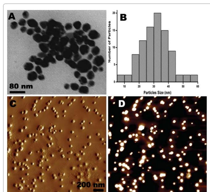
**Figure 1:** Transmission electron microscopy (A), and atomic force deflective (C) and topographical (D) images of the as-prepared parent silver nanoparticles suspension showing the anisotropic size and shape distributions of nanoparticles. (B) Surface height measurements obtained from the TEM image by counting ~100 particles.
