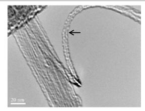
Figure 1: High-resolution transmission electron micrograph of SWCNTs. A representative crystalline structure of a bundle of SWCNT from HRTEM. Arrow shows the distinctive single-walled nanotubes structure (two tubes bound together with each diameter about 2 nm).
