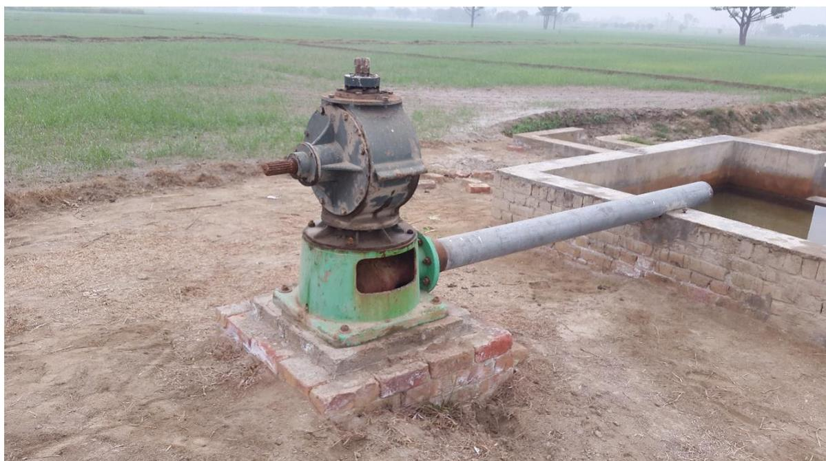
Figure 4: Turbine pump with PTO arrangement in Chak No. 60/12L in Bari Doab Region.
