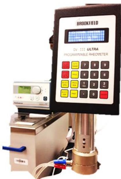
Figure 1: Wells-Brookfield cone-and-plate rheometer.
