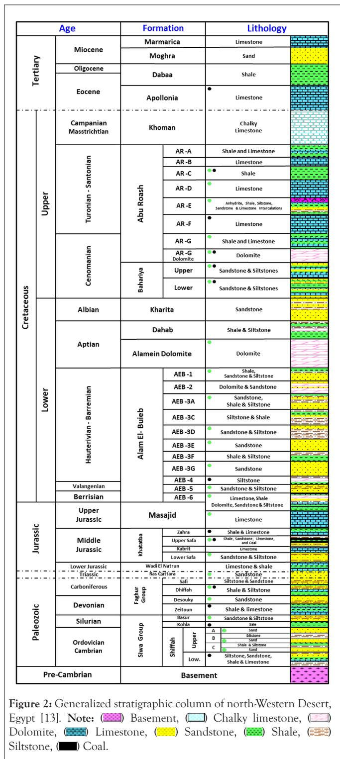
Figure 2: Generalized stratigraphic column of north-Western Desert, Egypt [13]. Note: (purple) Basement, (light blue) Chalky limestone, (pink) Dolomite, (blue) Limestone, (yellow) Sandstone, (green) Shale, (grey) Siltstone, (black) Coal.
