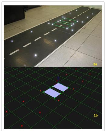
Figure 2: Markers placed along the walkway for kinematic recording. Each camera was positioned so as to offer optimal visualization of the markings on the floor, shaping the data collection walkway. 2a: Positioning of the markings on the floor. The dotted lines in the center of the walkway connect the vertex markings of the force platform. 2b: 3D imaging of the illuminated dots captured by the set of cameras.
