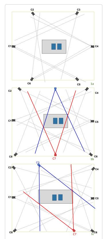
**Figure 1: 1a** –Positioning of 6 cameras equidistant to each other. Note the length and width of the recording area. **1b** – Length and width of the recording area with 8 cameras in the same positions as in 1a. **1c** – Positioning of the cameras with the goal of achieving optimal visualization of the entire central area of the study room. Both useful length and width increased considerably.
