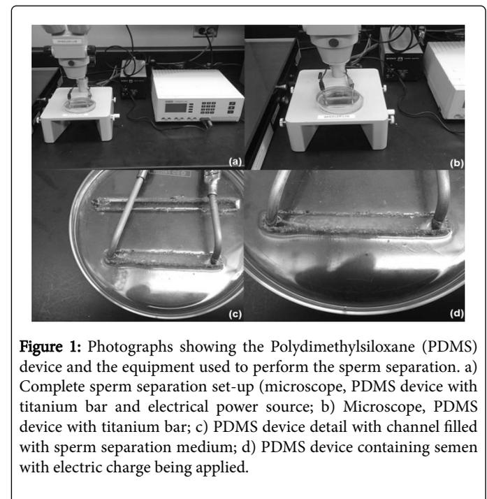
**Figure 1:** Photographs showing the Polydimethylsiloxane (PDMS) device and the equipment used to perform the sperm separation. a) Complete sperm separation set-up (microscope, PDMS device with titanium bar and electrical power source; b) Microscope, PDMS device with titanium bar; c) PDMS device detail with channel filled with sperm separation medium; d) PDMS device containing semen with electric charge being applied.
