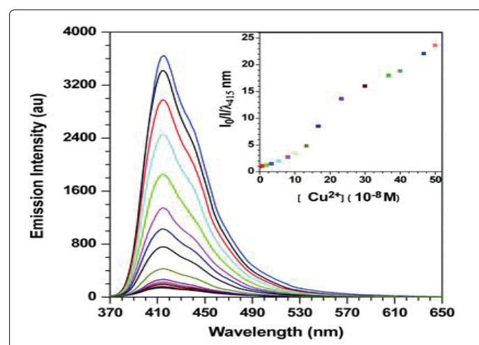
Figure 2: Calibration graph of  $Cu^{2+}$  - DNA/RNA chelate.
