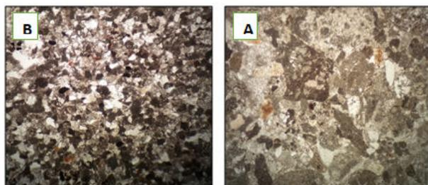
Figure 4: Microscopic Image of Bakhtiari Formation sediment (Source Rock of Studied Sediments) at 25 Magnification.
