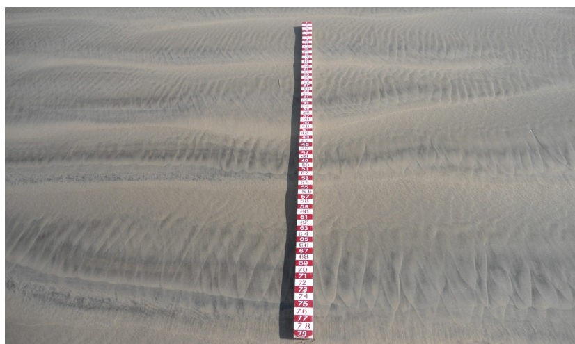
Figure 9: Sinusoidal wave sedimentary marks on the shoreline at 500m away from the estuary mouth at the updrift.
