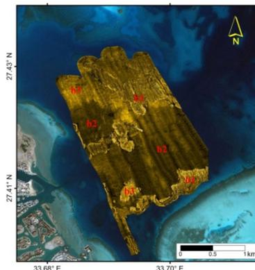
**Figure 7:** The side scan sonar mosaic map of El-Gouna Bay; (pattern with isolated reflections (b1), pattern of weak backscatter (b2) and pattern of strong backscatter (b3)).
