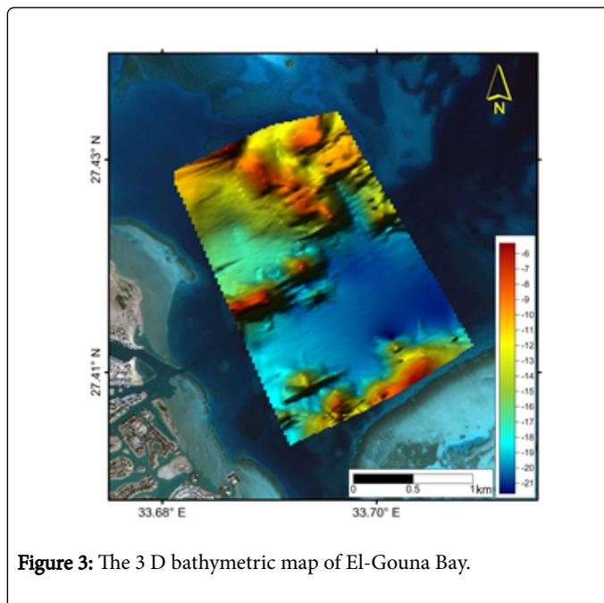
**Figure 3:** The 3 D bathymetric map of El-Gouna Bay.
