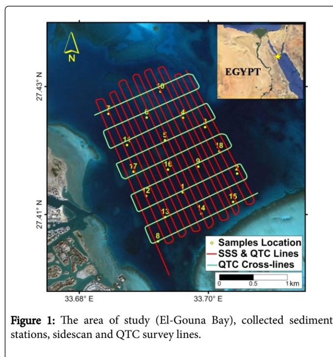
**Figure 1:** The area of study (El-Gouna Bay), collected sediment stations, sidescan and QTC survey lines.
