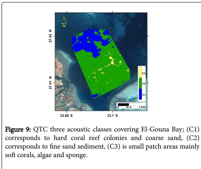
Pattern C1 from QTC is corresponding to both b1 and b3 from SSS. The single beam QTC system was unable to differentiate between the two patterns. While, the pattern C2 is corresponding to b2 that represent the fine sand sediments. On the other hand, QTC was able to detect a different signal corresponding to the soft bodies as soft corals, algae and sponges but in low resolution due to the single beam used.
