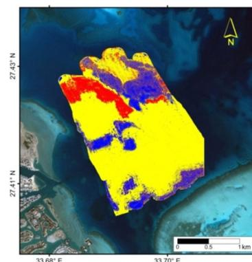
**Figure 8:** Post-processing for backscatter mosaic map by using the 'Extract Beam Pattern' along the study area: red colour indicates hard corals with coarse sand, blue color indicates soft corals and yellow colour indicates very fine sediments.
