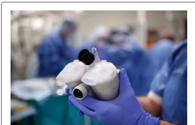
**Figure 2:** SRH11 prior to the implantation. Two pumps are coupled together to create the total artificial heart.
