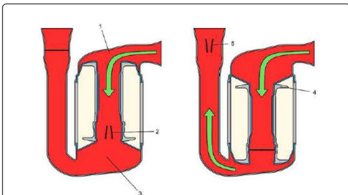
**Figure 1:** Prototype SRH11. A) Cross-section of a pump. Left: The diastolic phase. Blood enters the pump through the atria (1), passes the open bileaflet valve in the AV-plane (2), and fills the ventricle (3). The outflow valve is closed. Right: The systolic phase. The AV plane containing the valve (4) moves downwards, the AV-plane valve closes due to the increased pressure in the ventricle, and the blood is ejected through the open valve in the outflow cannula and the valve(5).
