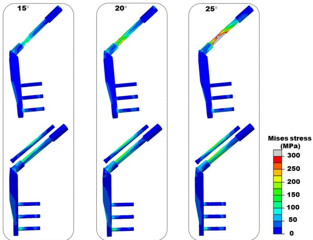
Figure 2. The stress distribution of CHS system with different operations in initial postoperative stage of osteotomy.
