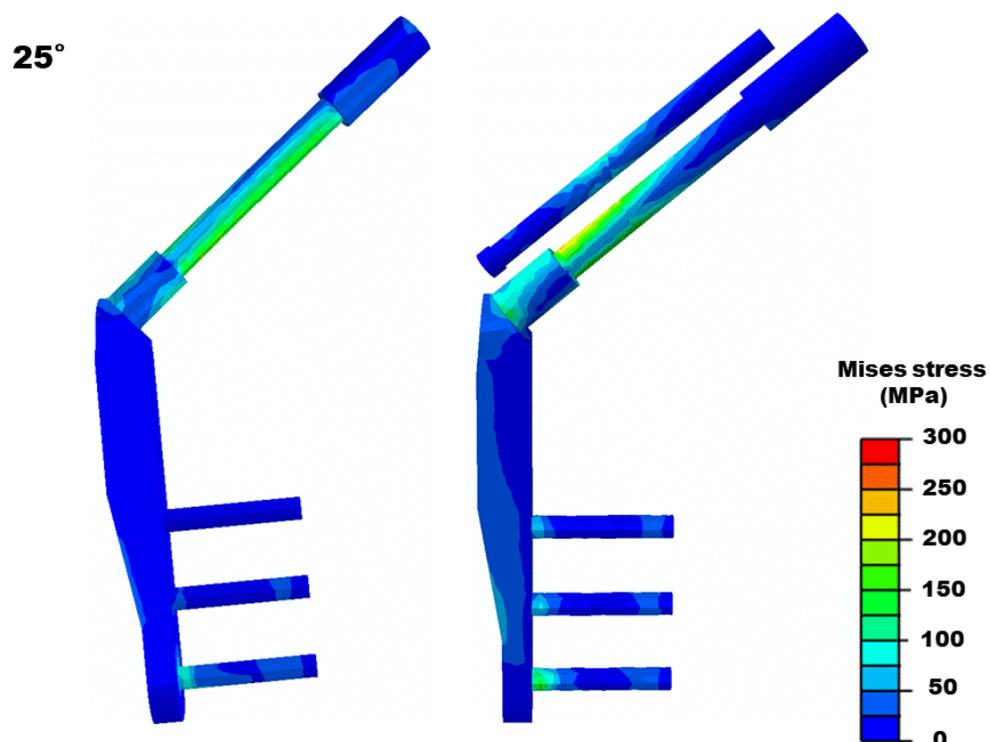
Figure 3. The stress distribution of CHS system of 25° CVO in bone-healing stage of osteotomy.
