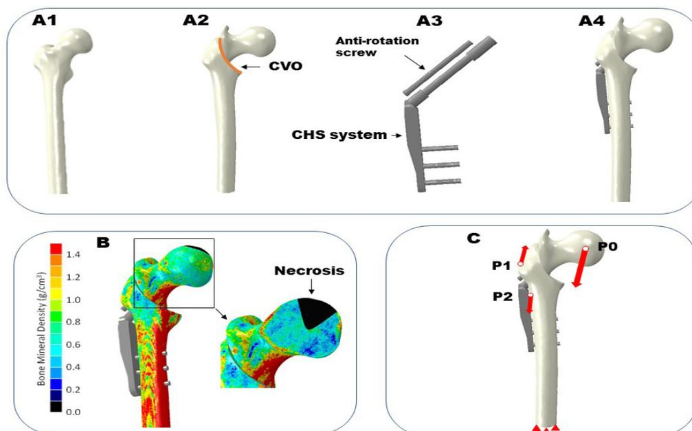
**Figure 1.** Reconstruction of CVO finite element model; A1): Intact femur 3D model; A2): Intertrochanteric curved varus osteotomy; A3): CHS system with anti-rotation screw; A4): CVO complex fixed with CHS system and anti-rotation screw; B): Femoral bone was assigned with isotropic elastic heterogeneous material properties; C): CVO finite element model with loading conditions.
