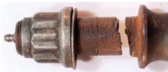
Figure 4: Corrosion at fracture site.
