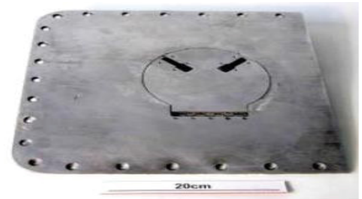
Figure 6: Wing panel and door outer surface after removal of catches and paint stripping.
