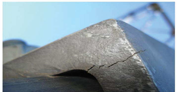
Figure 1: Material failure due to crack initiation.
