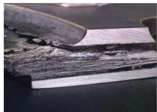
Figure 8: Cross section of panel showing Exfoliation corrosion.
