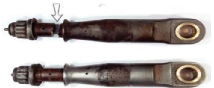
Figure 2: Broken steel pin of main landing gear.
