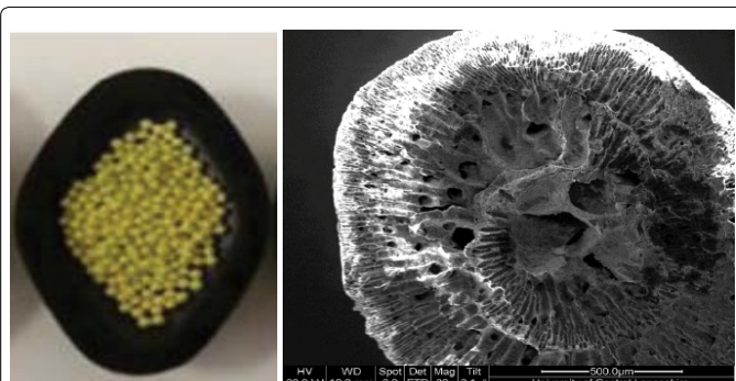
Figure 4: (a) AMP 50% PAN spheres. (b) SEM image of AMP (50%) PAN composite.
