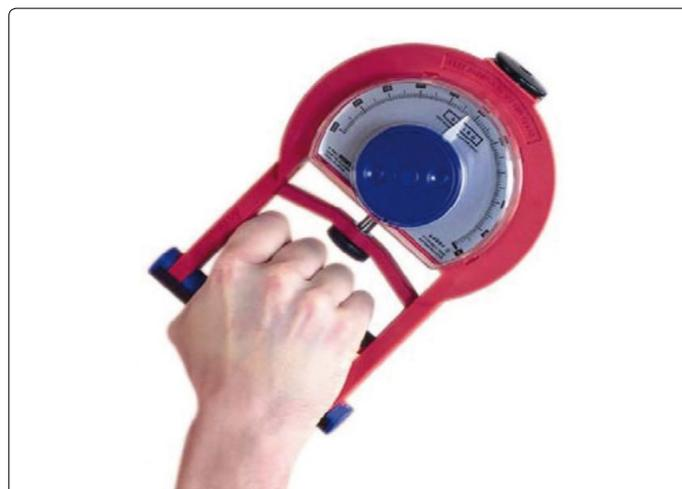
Figure 4: Dynamometer used in the handgrip force experiment.
