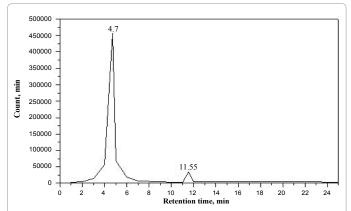
**Figure 6:** HPLC radiochromatogram of  $[Tc(CO)_3(H_2O)_3]^*$  precursor, pH = 11, flow rate 0.6 ml/min, R<sub>t</sub> = 4.5 min for  $[Tc(CO)_3(H_2O)_3]^*$ , R<sub>t</sub> = 11.44 min for free <sup>99m</sup>TcO<sub>4</sub><sup>-</sup> using 0.22 µm millipore filtration to eliminate unknown radiochemical impurities.
