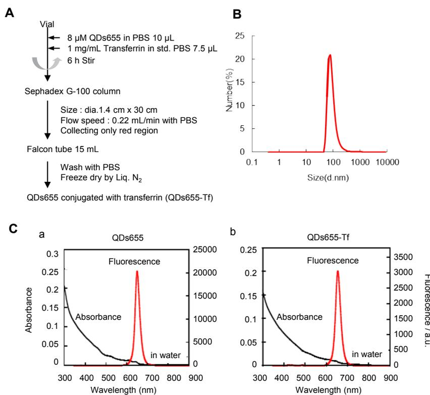
**Figure 2:** Synthesis and characterization of QDs655-Tf. (A) A scheme of the synthesis and column filtration of QDs655-Tf. (B) The size distribution QDs655-Tf in water. The peak size of QDs655-Tf was approximately 90 nm. (C) The absorbance and fluorescence spectra of QDs655 and QDs655-Tf in water.
